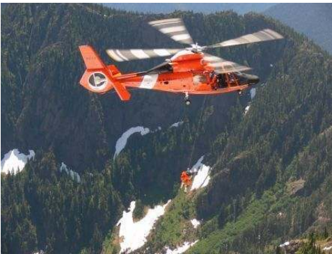
An HH-65C flight crew assigned to Coast Guard Air Station Port Angeles, Wash., hoists an injured hiker to safety from a mountain peak at an altitude of 6,300 feet--and a density altitude approaching 9,000 feet--in July. The rescue would have been impossible with the older, under-powered Bravo model. (Photograph courtesy of Brian "Red" Anderson)
